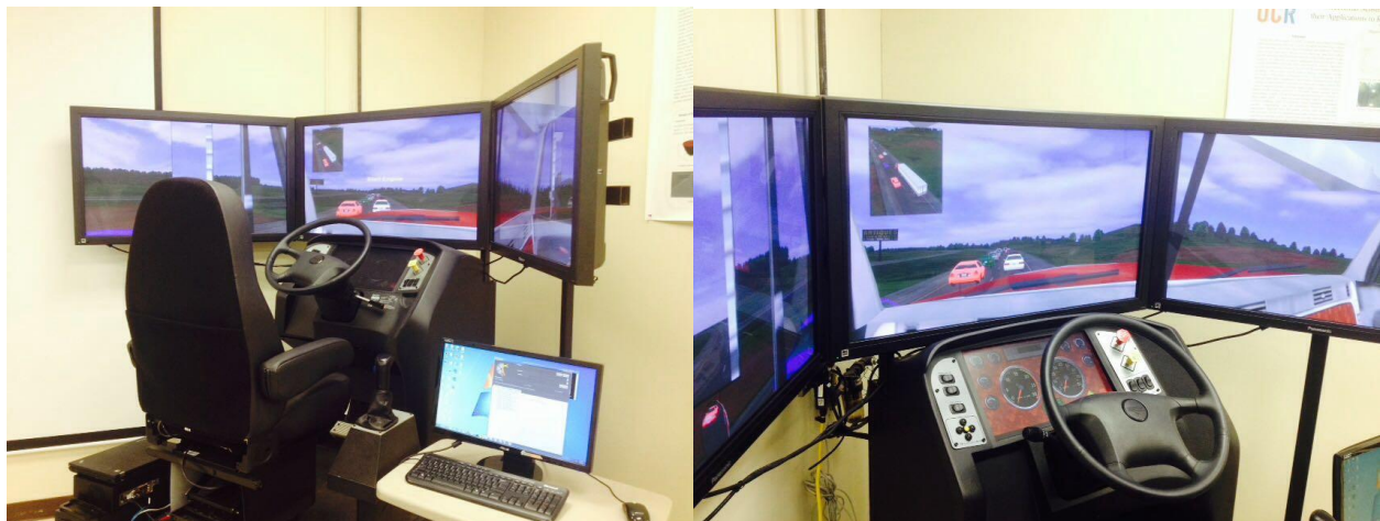
Figure 11. Minisim™ truck driving simulator at UCR
