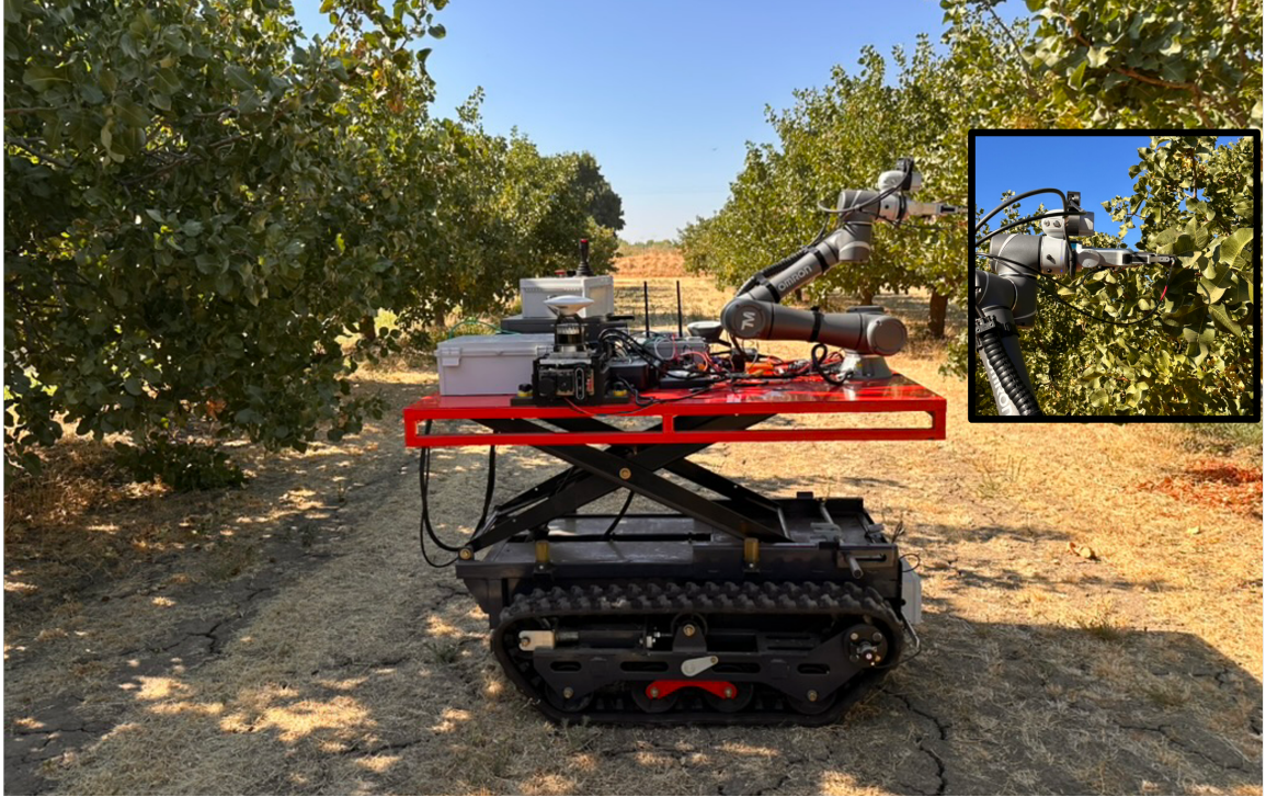
Figure 2.3: RoMu40, a robotic manipulation unit for orchard operations effectively automating ground-based crop mintoring and hyperspectral leaf sensing.
