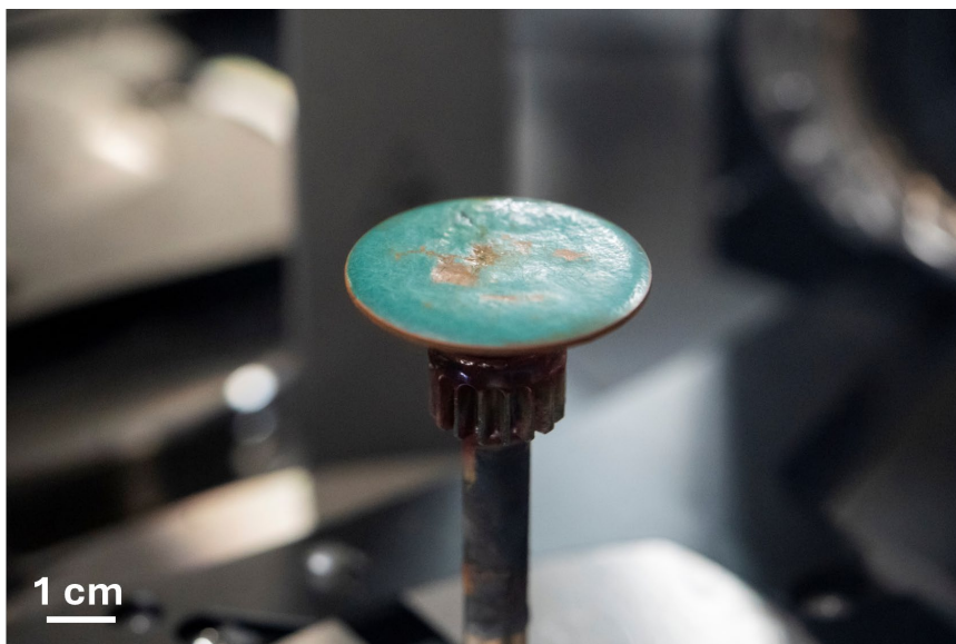
Figure 13. UZrFNaBe cooling on the lower parallel measuring plate after viscosity measurement. (Adam Lau/University of California Berkeley Engineering)
