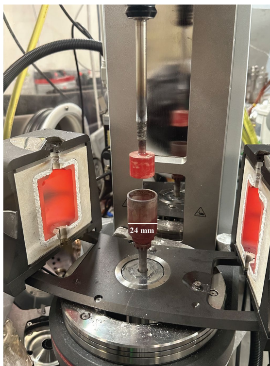
Figure 25. Image of rheometer with Inconel cup and bobber attached located inside of the argon glovebox post NaCl–KCl salt measurement.
