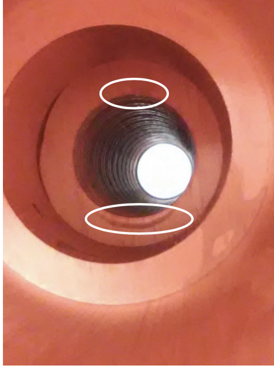
Figure 5.14: Photograph of the 3D printed, copper plated MTM SWS following 100 shots. Minimal damage was noted at the inlet (highlighted by the white ovals).
