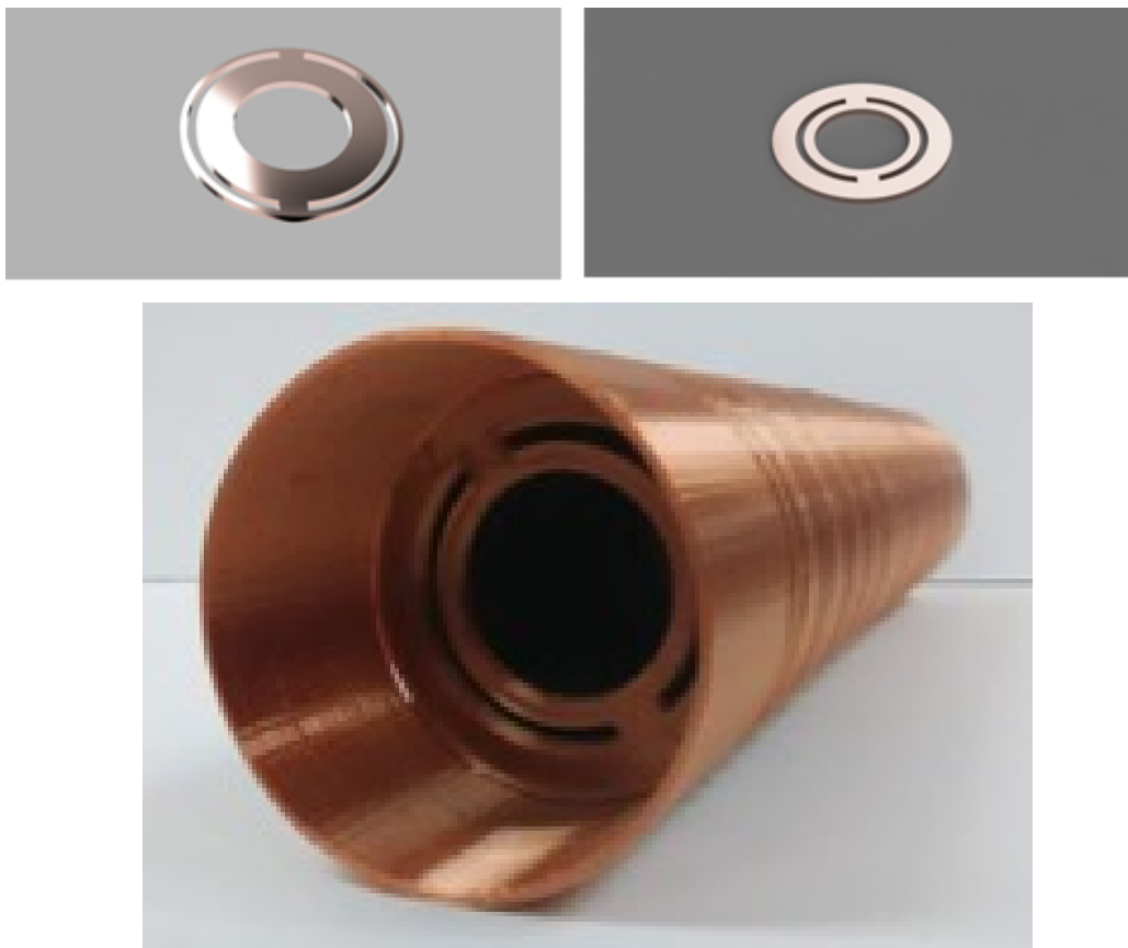
Figure 5.13: (Top) CAD drawing the two CeSRRs comprising a unit cell of the MTM SWS. (Bottom) 3D printed cylindrical tube housing the 11-cell MTM SWS.
