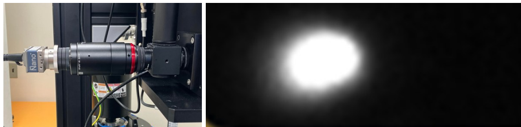
Figure 4.5. Coaxial camera and sample signal output with 8um pixel size
