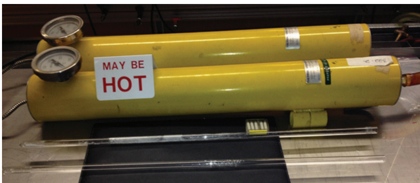
Figure 4.2: Thermal gradient sublimation apparatus with glass sublimation tubes containing biphenyl and pentaerythritol in the foreground.
