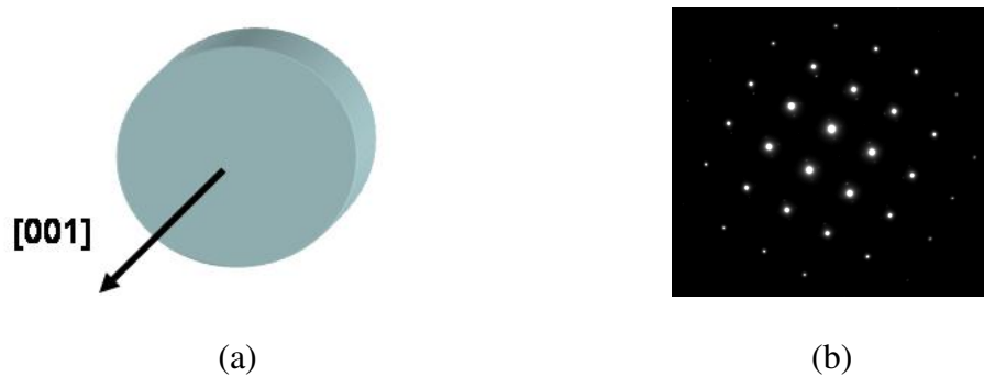
Figure 3.9: (a) [001] orientation of all samples. (b) Typical diffraction pattern of samples indicating the [001] orientation.
