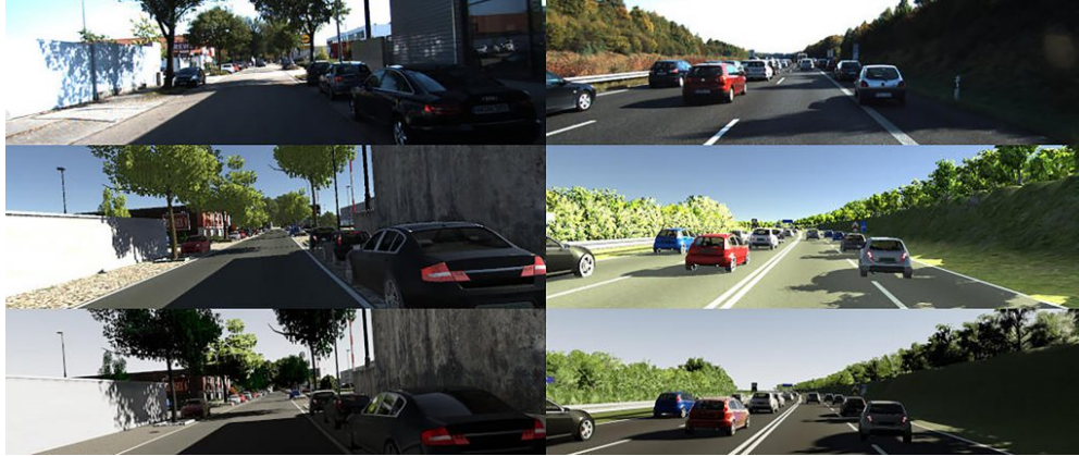
Figure 3.3: Example images from the original KITTI (top), Virtual KITTI (middle), and Virtual KITTI 2 (bottom) datasets, where we can notice the photorealistic rendering and the rendering style difference.
