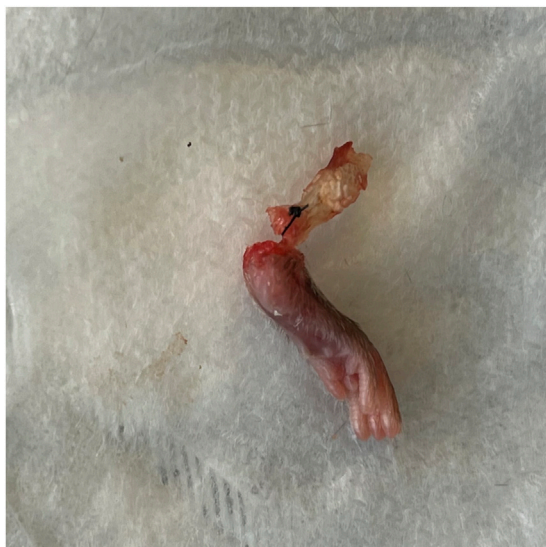
FIGURE 2 Representative specimen after load to failure. All specimens failed at the junction of the tendon/repairative tissue and bone.
