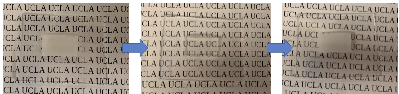
Figure 2-19. The demonstration of a complete transition process of a 1 mm thickness smart window film used ethanol as the solvent.
