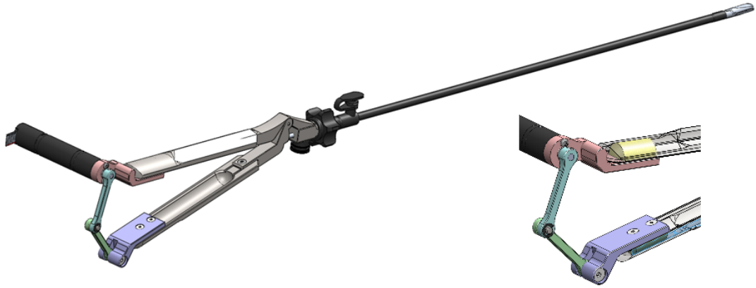
Figure 4.14: Four-Bar Mechanism CAD Model for the Karl Storz 33XXX CLICK'line Laparoscopic Instrument Series
