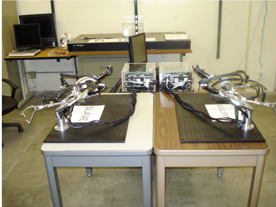
Figure C.21: LapaRobot 2.2 Master/Slave Surgical Stations Prototype, Side View
