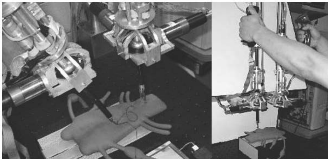
Figure 1.6: The Endobot, or Robot Assisted Suturing and Automation System [16]
