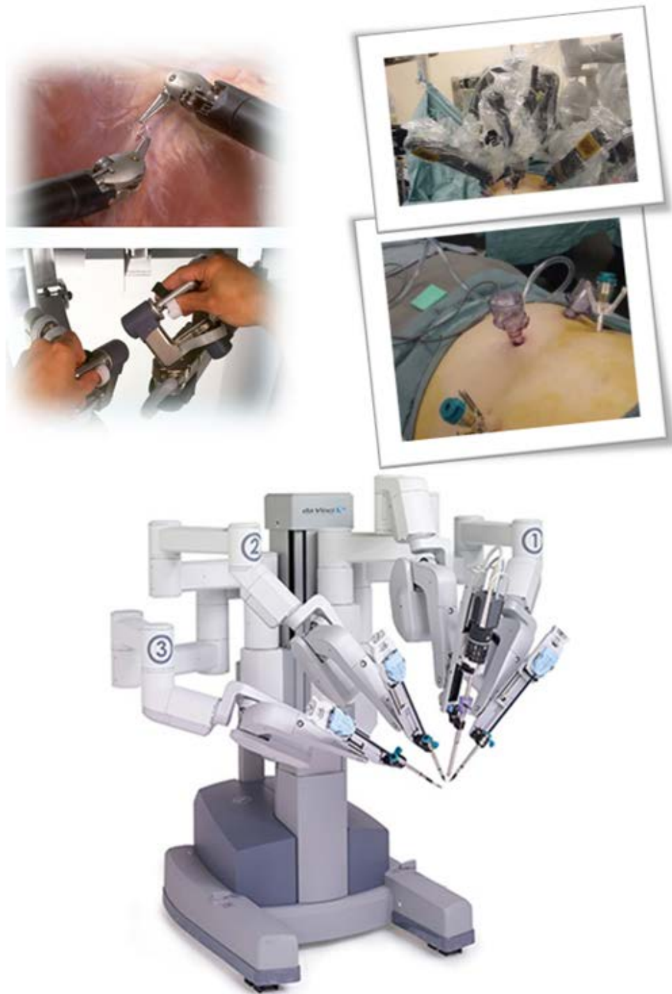
Figure 1.4: The da Vinci Surgical System by Intuitive Surgical Inc. [18]
