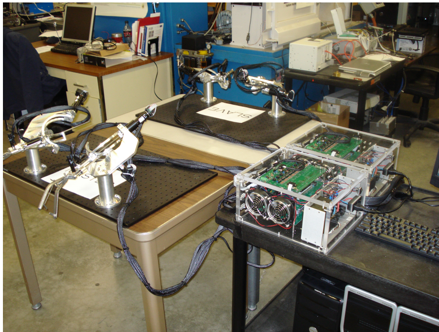
Figure C.20: LapaRobot 2.2 Master/Slave Surgical Stations, Prototype
