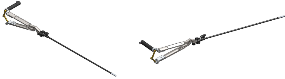
Figure 4.20: Four-Bar Mechanism CAD Model for the Karl Storz 33XXX CLICK' line Laparoscopic Instrument Series (Left, Front Isometric View); (Right, Rear Isometric View)
