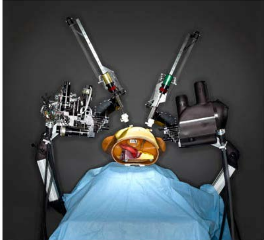
Figure 1.9: The Raven: A Surgical Robot System for Open and Minimally Invasive Surgery [24,25]
