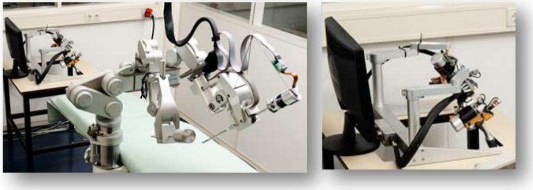
Figure 1.5: SOFIE: Surgeons Operating Force-Feedback Interface Eindhoven Robot [20]
