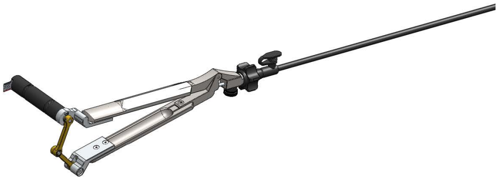
Figure C.10: Four-Bar Grasping Mechanism CAD Model, Isometric View
