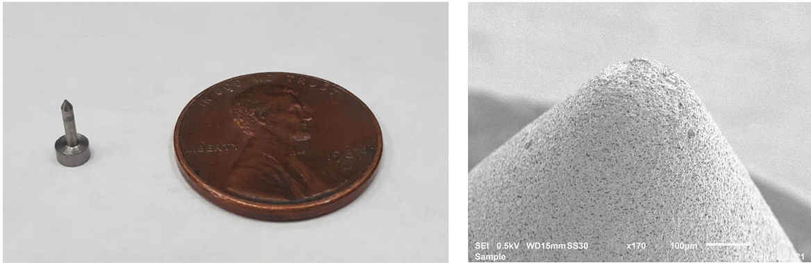
Figure 4.4: Left, conventionally machined porous tungsten emitter with US penny for scale. Right, SEM image of the emitter tip after electrochemical etching.
