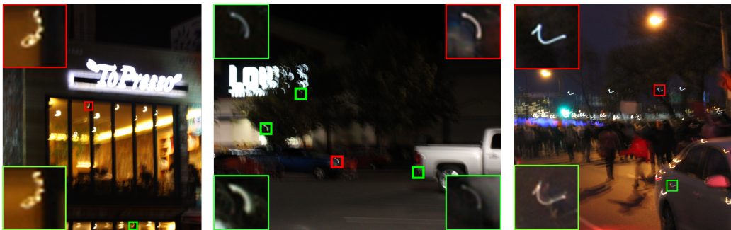
Figure 4.2: Examples of light streak detection. The red box indicates the best light streak patch and the green boxes show additional light streak patches that are automatically identified.
