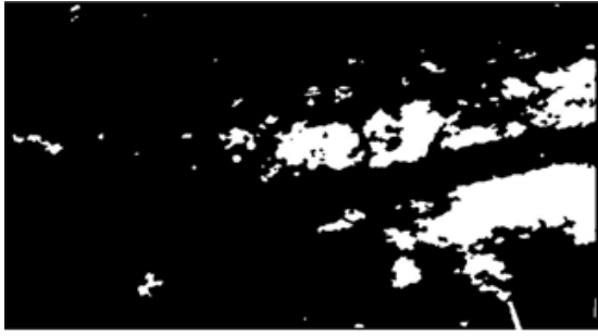
(a) Bi-level snapshot of the environment at 10:00 a.m. after applying a threshold to the segmented gray scale image
