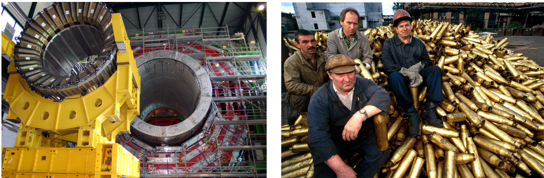
Figure 2.13. A photograph of the CMS hadronic calorimeter (HCAL) in front of the magnet and muon chambers before the detector was installed in the experiment cavern (left), from Ref. [87], and workers in Mormansk sitting on the decommissioned World War II artillery shell casings used to supply the brass for the HCAL (right), from Ref. [88].
