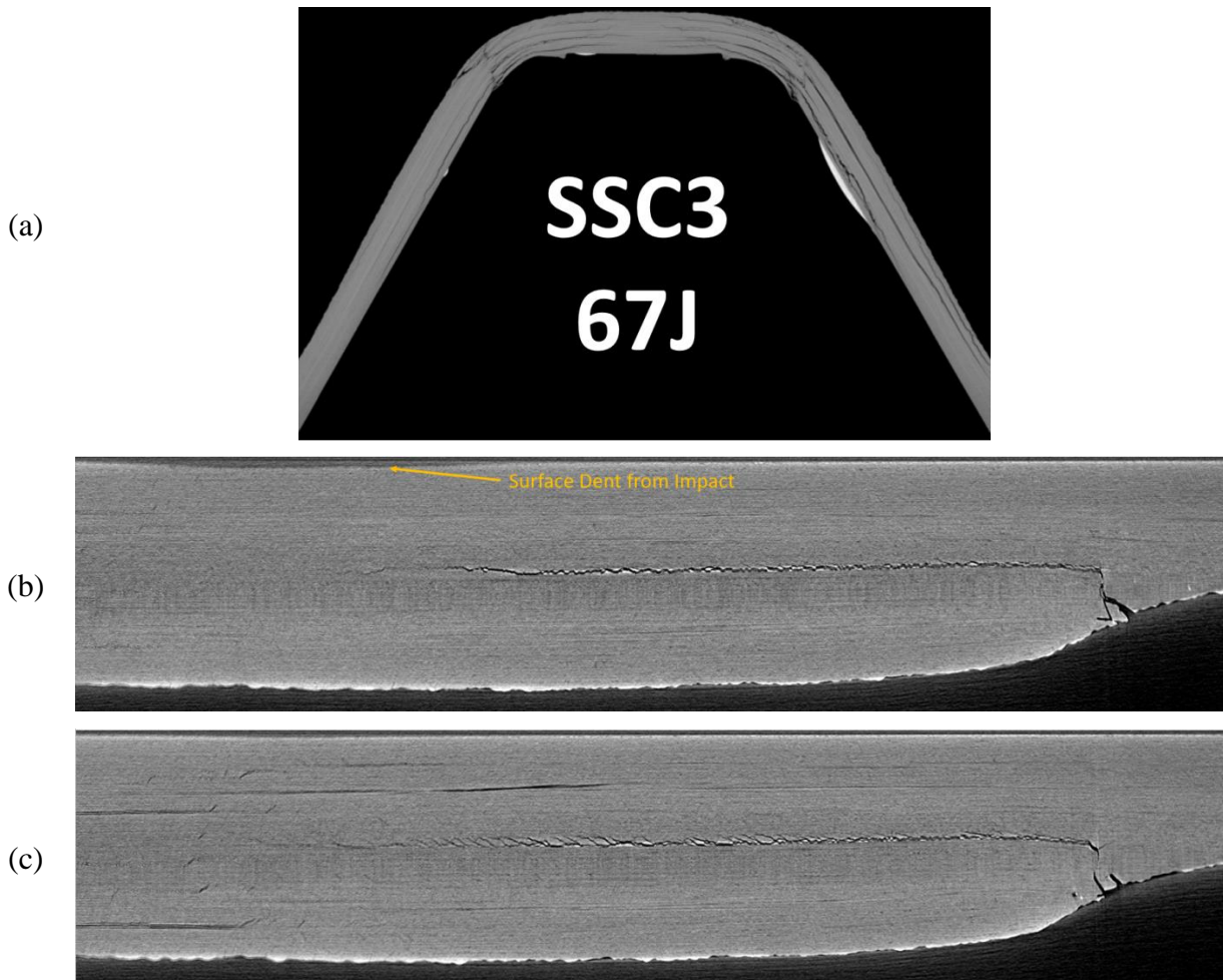
Figure 3.2.2.4. Cross-sectional CT scan image of the (a) 67 J cap-impacted SSC3, and (b) 65 J flange-impacted S4F1 at COI and (c) 1.5 cm away from COI [30]
