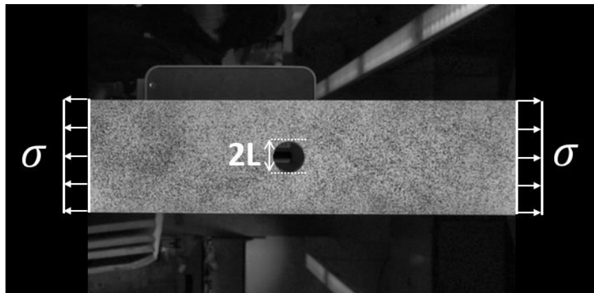
Figure 4.1.1. OHT tension test coupon with DIC speckle pattern
