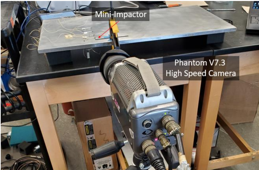
Figure 2.3.1.2. Mini-impactor test with high-speed camera
