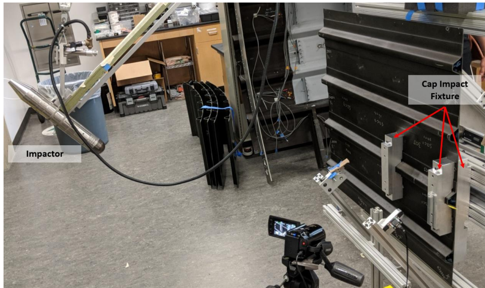
Figure 3.2.1.2. Pendulum impactor setting for the cap impact at region S3C1 for 30 J target impact
