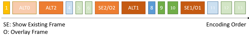
(b) Symmetric multi-reference prediction in encoding order (SE for non-filtered ALTREF_FRAMES and O for filtered ones)
