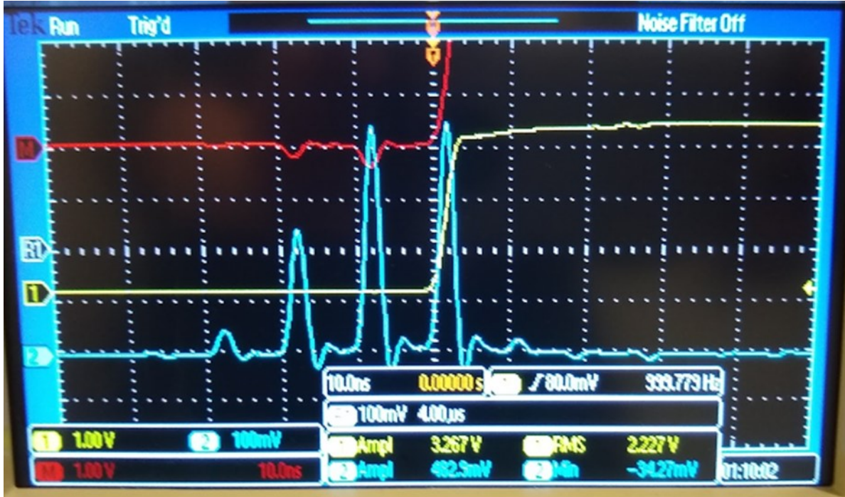
Figure 3.4. Example of the amplification build-up of a well-aligned regenerative amplifier is shown in the blue oscilloscope trace. A photodiode is installed behind one of the cavity mirrors, measuring the leak through of the seed pulse as it travels through the cavity. Only the last 4-5 pulses have sufficient intensity to be measured. Each round trip is separated by \sim 9 ns.
