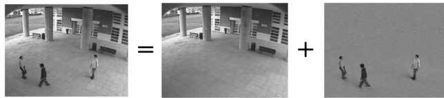
Figure 3.10: Sample output of Robust PCA for stationary video background subtraction. Video is from the ViSOR surveillance video database [93].
