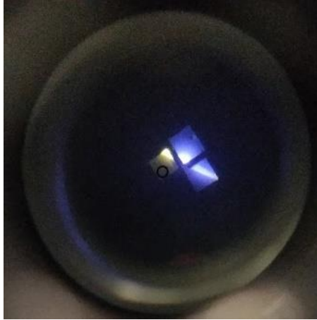
Figure 2.11 LED samples showing emission under RHEED at the initial stage of growth. The blue samples were LEDs. The yellow sample was GaN on sapphire template.
