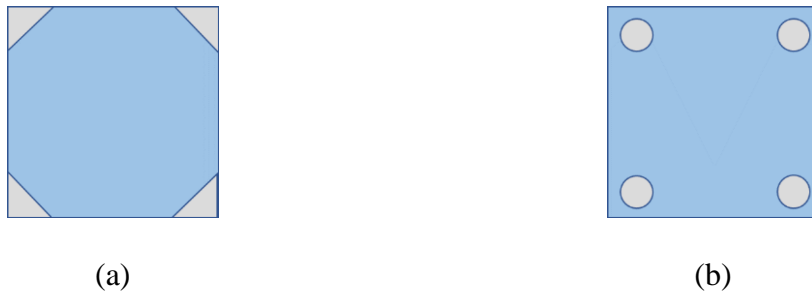
Figure C1. Indium dot Hall measurements where (a) the dots are put on the corners (b) the dots are put within the sample border.
