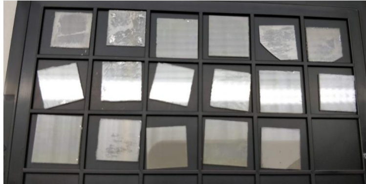
Figure 2.10 Examples of samples with and without titanium backside coating grown with indium bonding. The indium and titanium on the sample backside partially evaporated during growth.
