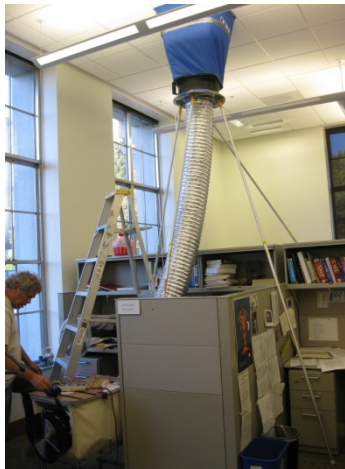
Figure 4.3-5 Apparatus for Measuring of Actual Airflow from Diffusers
