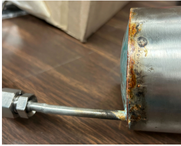
Figure 4d shows oxidation at the bottom of the cup due to low temperature.
