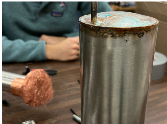
Figure 4a shows the copper wires on the cold head (left) and the damaged cup (right). Oxidation can be seen on the copper plates.
