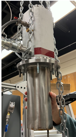
Figure 4b shows the cup-cryocooler assembly taken out of the condenser.
