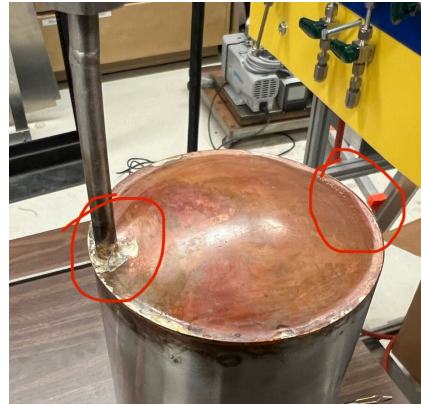
Figure 4e shows the leak point, marked with a red circle.
