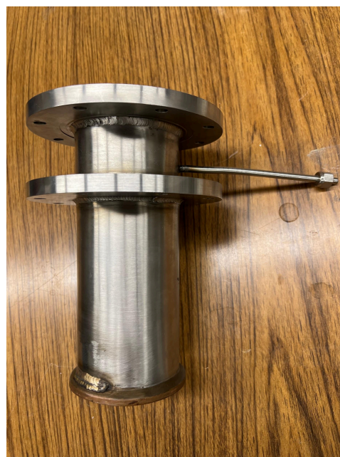
Figure 5b shows the cup after use. The copper plates on the bottom were removed.
