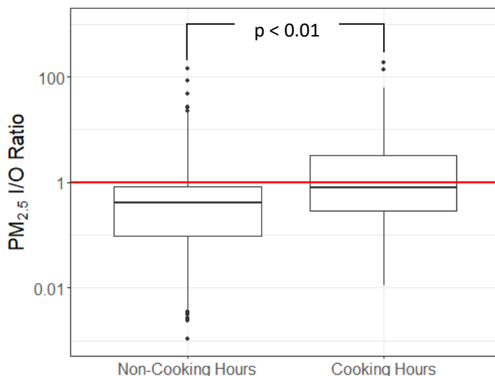
Figure 3. Log-scale PM_{2.5} I/O ratios during cooking and non-cooking hours. The solid horizontal line represents the median. The box represents the 25 th to 75 th percentiles, and the whiskers represent the outliers. The red solid line indicates where I/O ratio = 1.
