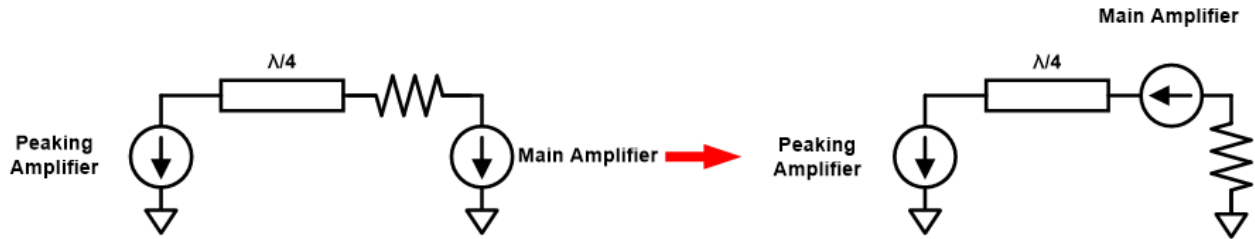
Figure 2.5: Transformation of the series DPA into a single-ended series DPA with the main and peaking amplifiers stacked.
