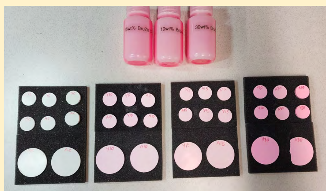
Figure 4. Non-sintered doped samples, with a darker pink color indicating a higher dopant concentration
