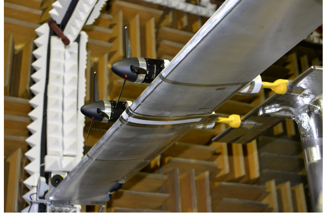
Figure 1: Experimental propeller-wing setup (Ref. 3). Note, the orientation of the wing in relationship to the propeller is inverted in the experiment as compared to Fig. 2.
