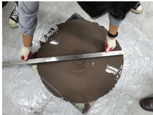
Figure 2. Flowability test of CLSM developed in this study.
