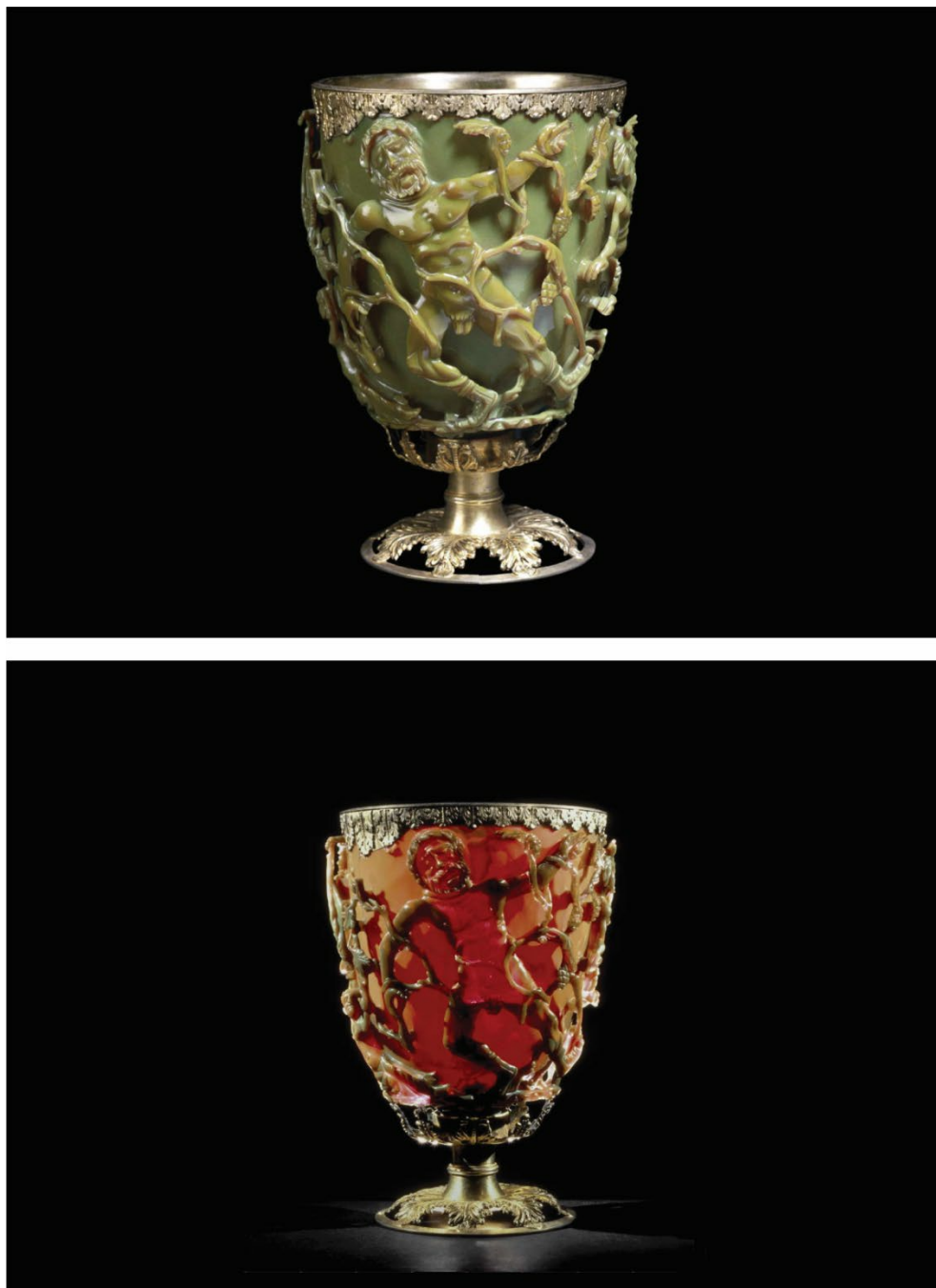
Figure 1.2. Photographs of Lycurgus Cup. The dichroic effects upon light irradiation from different angles are due to the gold and silver nanoparticle colorants. © The Trustees of the British Museum.
