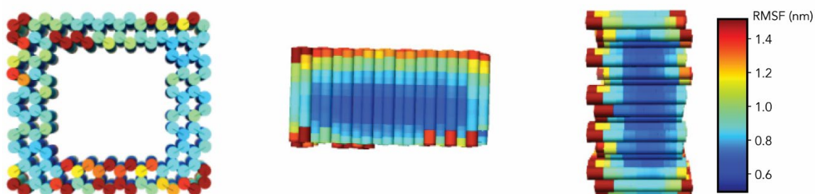
Figure A.1. CanDo simulation results. (a) Rothemund tile has maximum RMSFs value of 6.03 nm, and 95% red region (most flexible) RMSFs \sim 4.12 nm. (b) Our 3D DNA origami cage has maximum RMSFs value of 1.51 nm, and 95% red region (most flexible) RMSFs \sim 1.05 nm.
