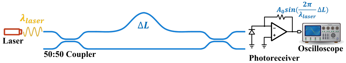
Figure 1.5: Basic block diagram relating the effect of a path difference to the interference pattern at the output
