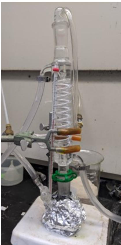
Figure A.4: Photograph of the reflux setup to dissolve 5g of V_2O_3 powder in 7M H_2SO_4 under flowing nitrogen.
