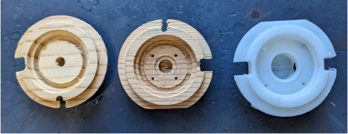
Figure 2.9: Three of the early machining tests, starting from wood (left, center) to HDPE (right).
