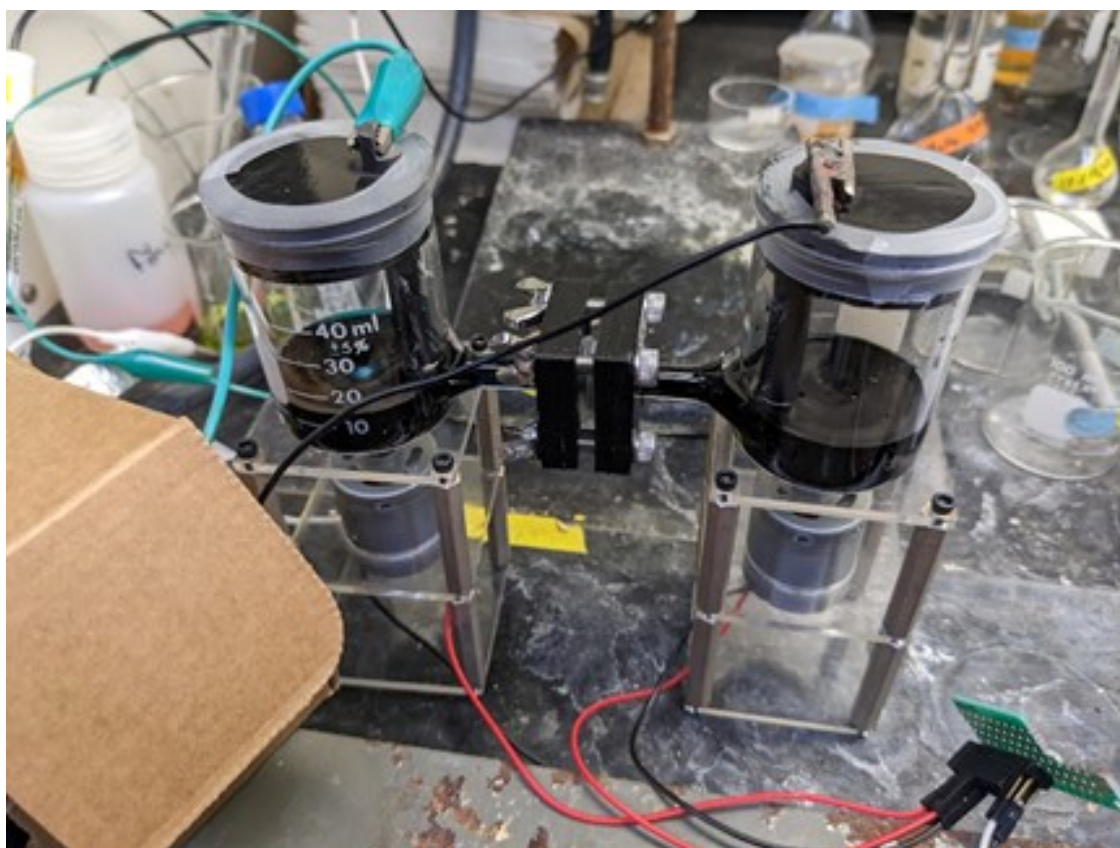
Figure A.9: Photograph of the fully assembled redesigned glass electrochemical cell, with both sides filled with electrolyte and with custom-built DC-motor magnetic stirrer plates..
