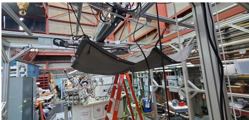
Figure 5.5. X-Y stages, source, and chopper installed on the mounting frame, along with an Eccosorb blanket to minimize stray reflections and pickup off the metal frame.
