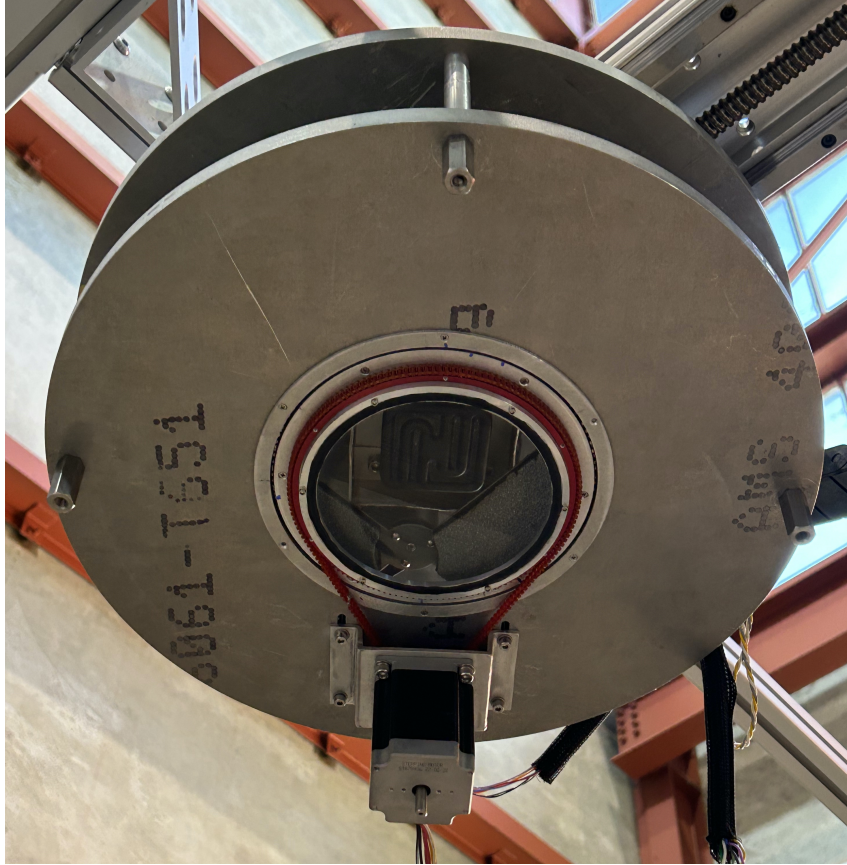
Figure 5.18. Stepped, polarizing grid installed in front of the thermal source and chopper. Not present in this picture: the 3.8-cm aperture to restrict reflections and systematics from appearing in the observed detector signal.
