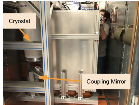
(b) Photo of the FTS on its cart with its coupling mirror installed. The full assembly is positioned next to the test cryostat.
