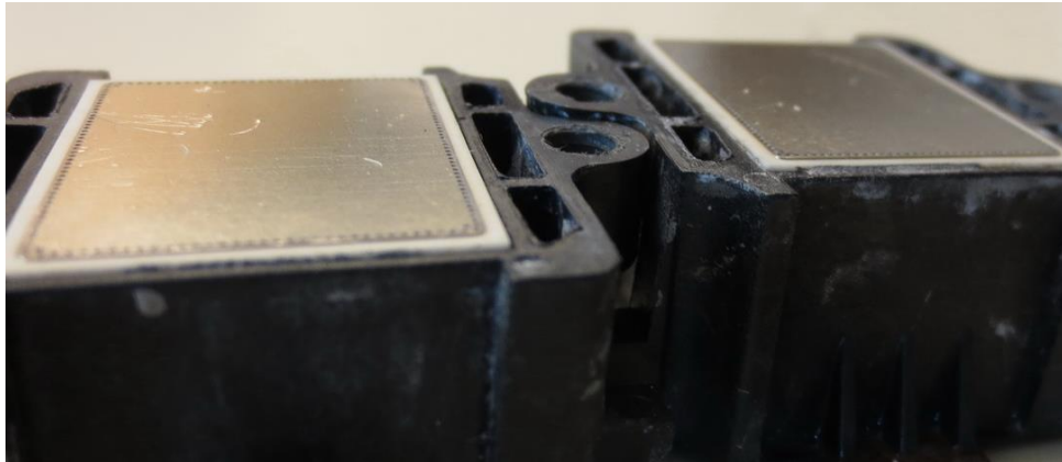
Figure 2.24: Contact surfaces can develop surface defects arising from continuous testing of the same heatsinks and back plates.
