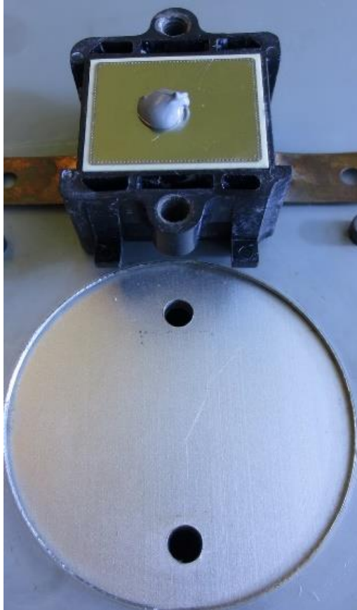
Figure 2.17: Example of application of thermal interface material.
