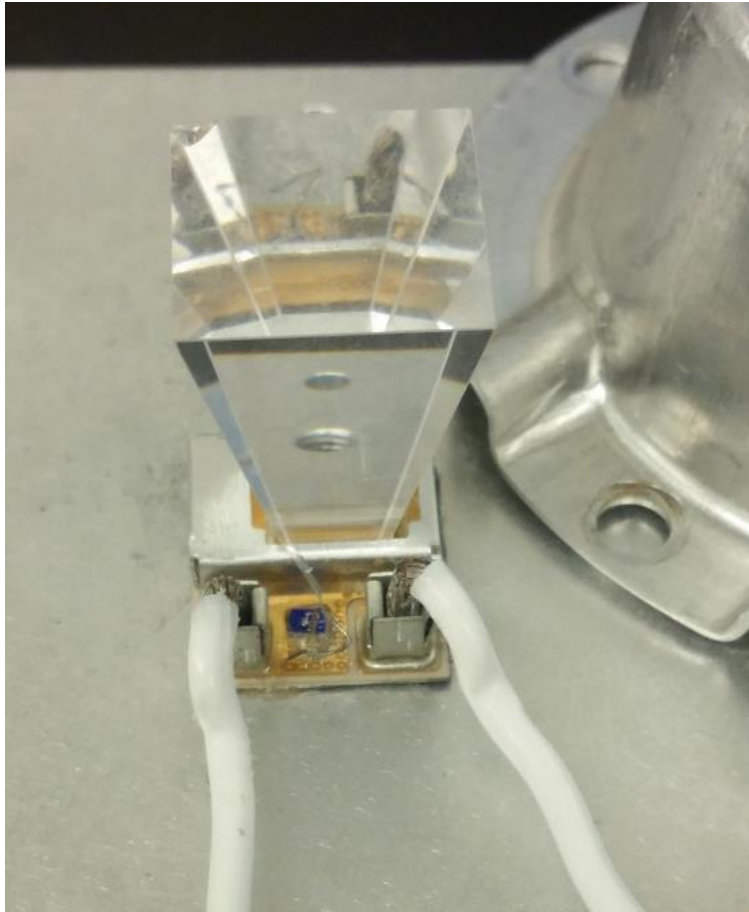
Figure 3.17: Multi-Junction solar cell with additional optical lens to achieve higher concentrations.
