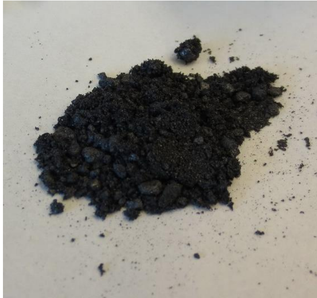
Figure 2.10: Optical image of graphene nanopowder with average thickness of 12 nm.
