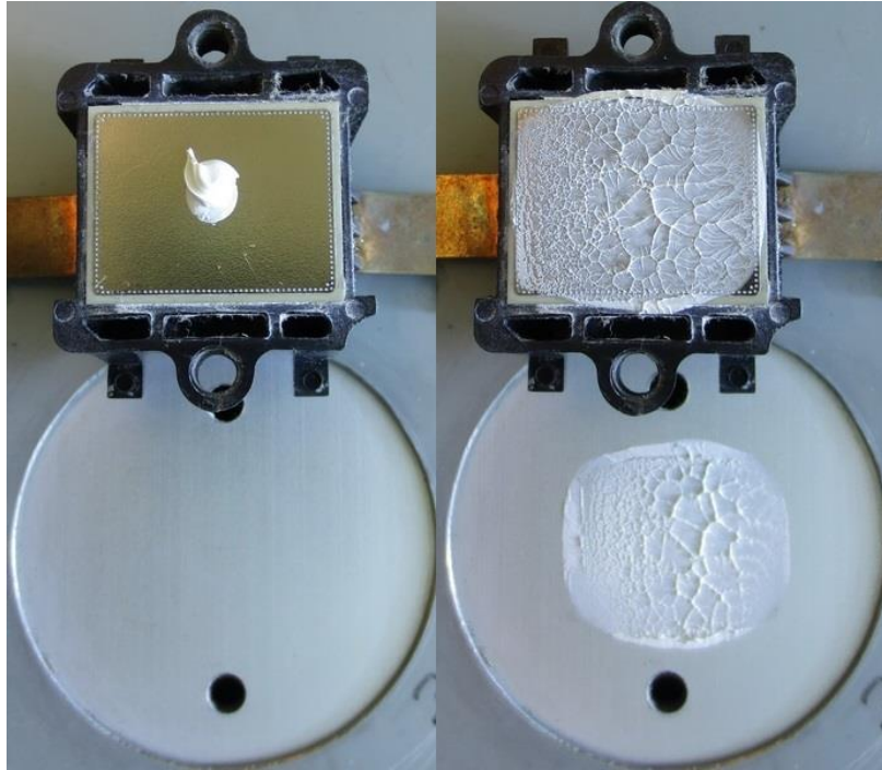
Figure 2.19: Typical spreading of thermal interface material.
