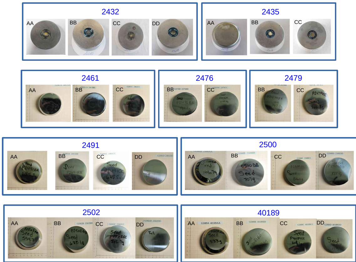
Fig. 1 Full inventory of crystal slices/diodes belonging to the GERDA Phase II BEGe detector production. Crystals/diodes obtained from the same ingot are framed in blue. The GD32 and GD35 detector series
