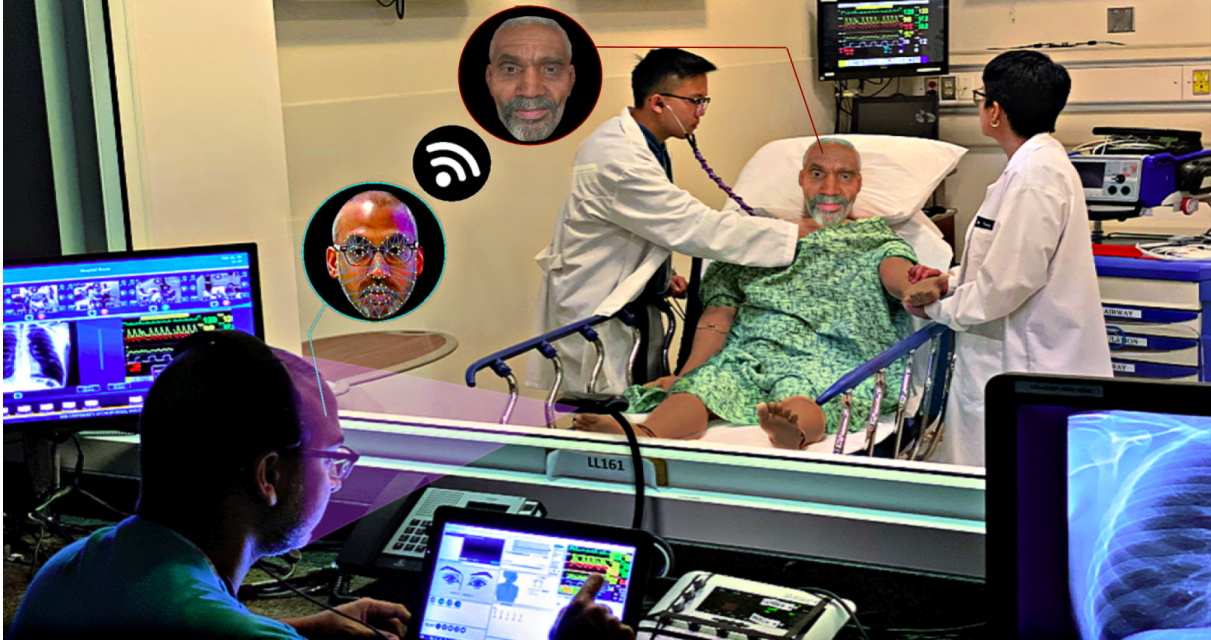
Figure 4.1. Robotic patient simulators are tele-operated, life-size mannequins that can exhibit thousands of physiological signals, and can breathe, bleed, and respond to medications. However, they are largely inexpressive, leading to poor training outcomes for CLs, and possibly poor clinical outcomes for patients. Our work addresses this gap by introducing patient simulator systems with a much wider range of expressivity, including the ability to express pain, neurological impairment (e.g. stroke, Bell’s Palsy), and other clinically-relevant expressions, via simulators with diverse genders, races, and ages.
