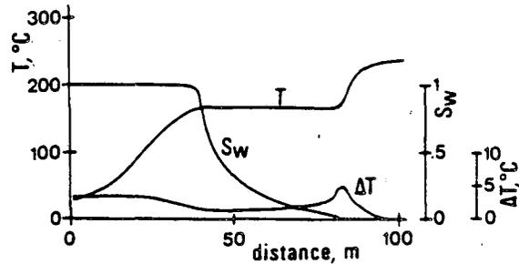
Fig. 7. One-dimensional radial, fractured-porous medium model (injection rate = 2.78 kg/s,  $k=5e-13 \text{ m}^2$ ). Variation with radial distance of temperature and liquid saturation in the fractures, and temperature difference between the outermost matrix elements and fractures.
