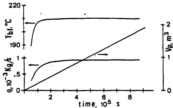
Fig. 2. One-dimensional, porous medium column. Production rate, boiling temperature and volume of liquid phase versus time for  $q_{inj} = 2.75e-3$  kg/sm<sup>2</sup>,  $k=5e-13$  m<sup>2</sup>.
