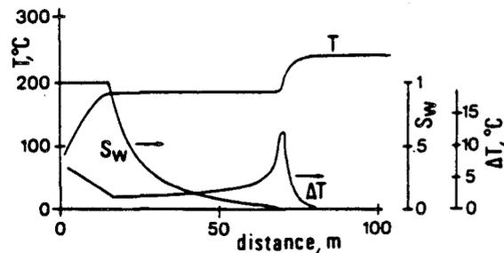
Fig. 5. One-dimensional, fractured medium column. Profiles of temperature and saturation in the fractures and temperature difference between outermost matrix elements and fractures for  $q_{inj} = 3e-4 \text{ kg/sm}^2$ ,  $k=5e-13 \text{ m}^2$
