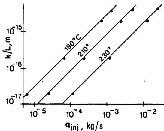
Fig. 3. One-dimensional, porous medium column. Dependence of stabilized boiling temperature on injection rate, permeability, and length of steam flow-path. Lines: from equations (1) to (3); solid circles: from numerical simulations.
