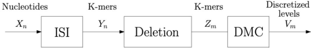
Figure 2.6: Simplified nanopore channel model from [2].
