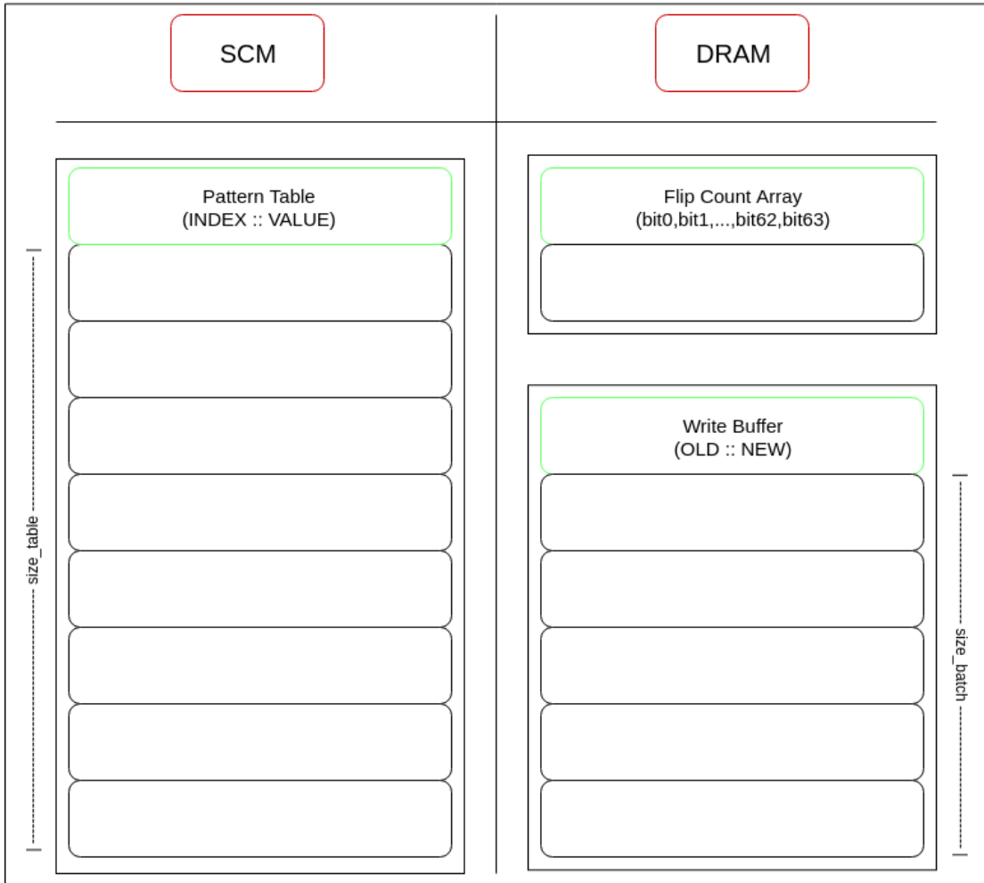
Figure 4.1: An overview of the main components of ABFPL and where they reside. In addition, an example with values from our simulation is shown in A.1
