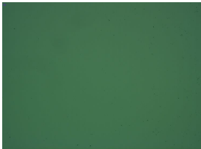
Figure 72 SI GaAs after annealing at 800 C with sputtered nitride as encapsulant
