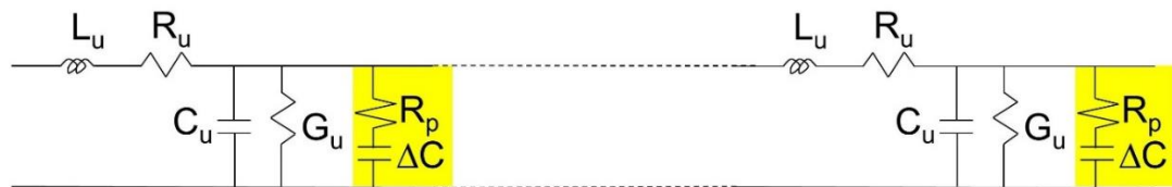
Figure 53 Electrical Loss simulation equivalent circuit
