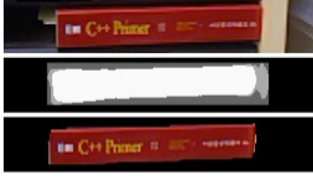
Figure 3: Top: a book as example object. Middle: initialization of GrabCut, the grayscale values correspond to the four possible likelihoods FG (white), PR\_FG (light gray), PR\_BG (dark gray), and BG (black). Bottom: the segmentation result.
