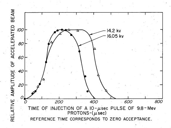
Fig. 2. Bevatron acceptance time for 16.05-kv and 14.2-kv magnet voltage. Conditions:
