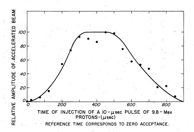
Fig. 3. Bevatron acceptance time for 8.03-kv magnet voltage. Conditions:
