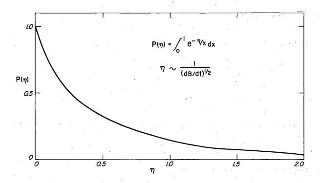
Fig. 1. Probability of an ion's missing the inflector as a function of the rate of rise of magnetic field.
