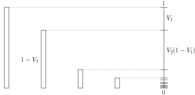
Figure 2.3: An illustration of how stick-breaking divides the unit interval into a sequence of probabilities (Broderick, Jordan, and Pitman, 2012). The stick proportions (V_1, V_2, \dots) determine what fraction of the remaining stick is appended to the probability sequence at each round.
