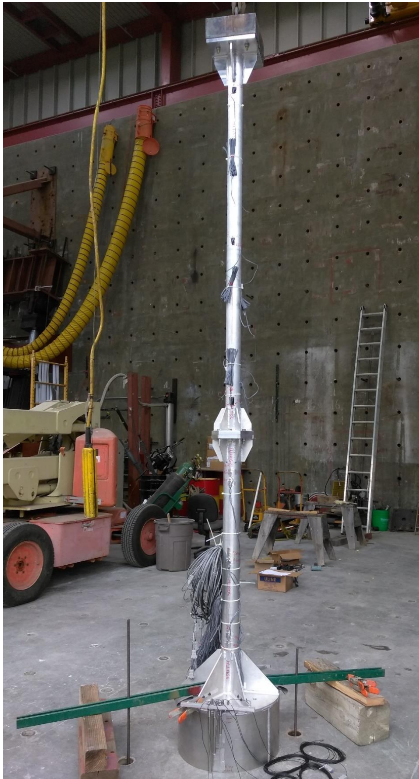
Figure 3-11: View of bucket foundation wind turbine model with fixed-base configuration before performing modal analysis for system identification
