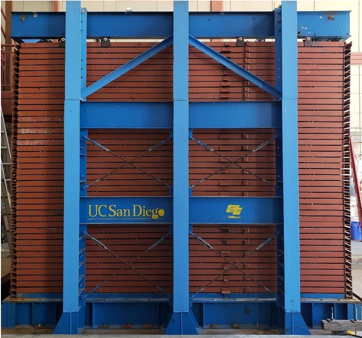
Figure 8-2: Laminar soil container with internal dimensions of 3.9 m x 1.8 m x 1.8 m (Length x Width x Height), placed on shake table at the UC San Diego Powell Laboratory
