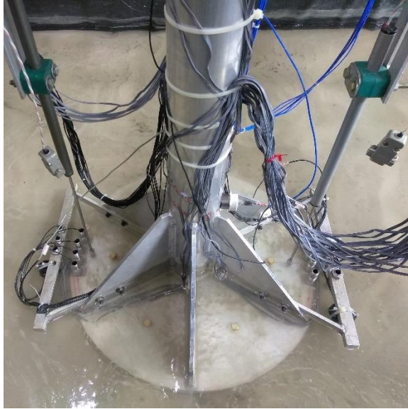
Figure 3-9: Bucket foundation after being installed in the saturated sand with instrumentation attached to it
