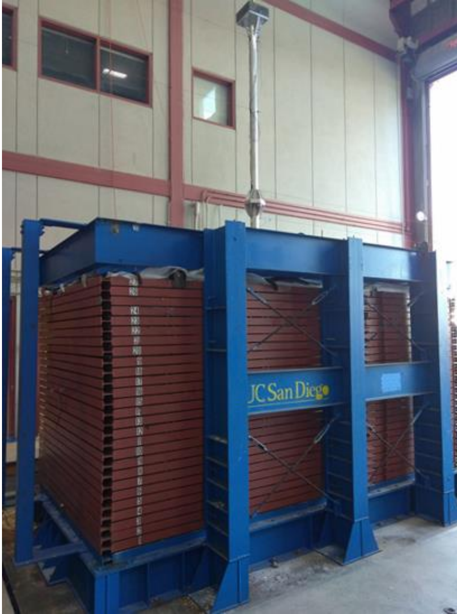
Figure 3-1: Laminar soil container placed on shake table at the UC San Diego Powell Laboratory
