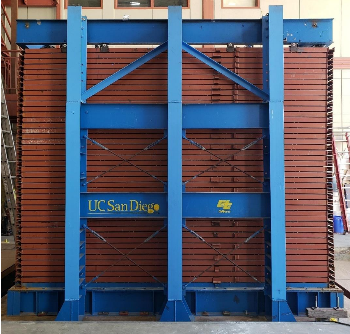
Figure 9-7: Laminar Soil Container Placed on Shake Table at the UC San Diego Powell Laboratory
