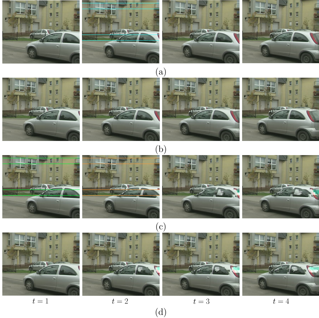
Figure 1.12: Channel distortion and error propagation for 3D video encoded using MVC. Reconstructed (a) primary view and (b) secondary view when no losses happen. Reconstructed (c) primary view and (d) secondary view when two slices are lost in primary view at t = 2 . Errors due to losses in primary view propagate to the frames of both the primary view and the secondary view.
