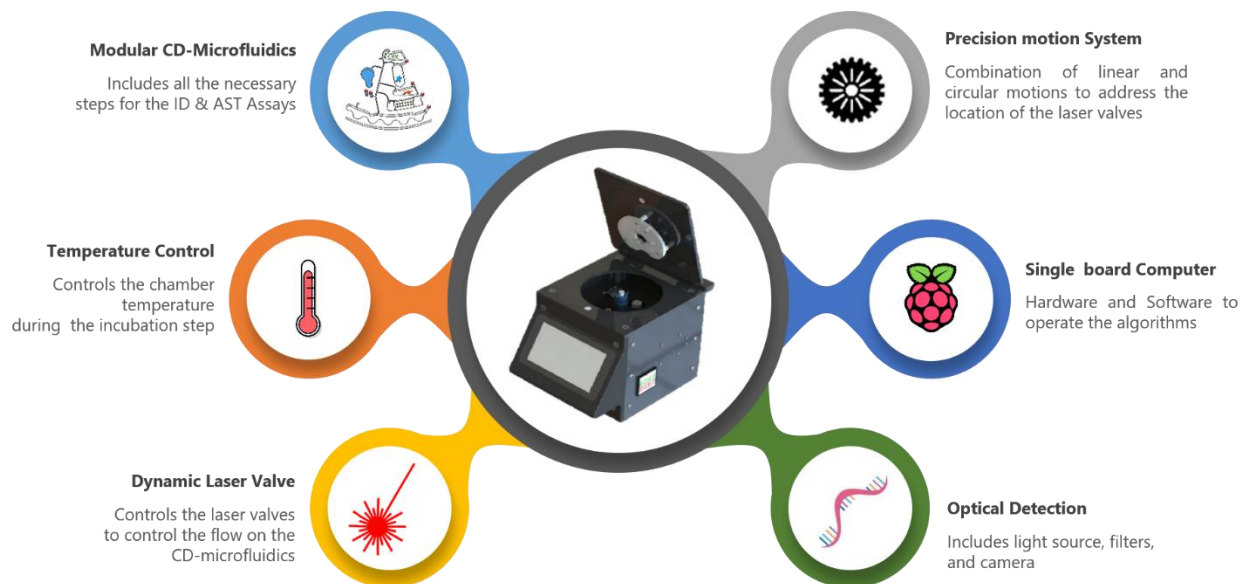
Figure 1.2. The SpinBox design and components.
