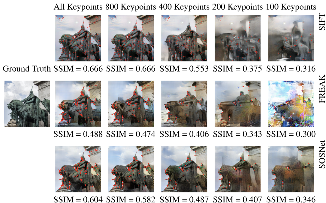
Figure 4.4: Reverse engineering ablation study of reducing keypoints. SIFT, FREAK and SOSNet reverse engineering results using 1,000, 800, 400, 200, and 100 keypoints respectively, annotated in red. Reducing keypoints reduces the potency of the reverse engineering attack. Regions with higher densities of keypoints have better reconstruction quality.
