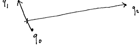
Figure 3.13 The Jacobi coordinates: Q_0 = q_0 and Q_1 = q_1 - q_0 and Q_2 = q_2 - \sigma_1 q_1 - \sigma_0 q_0 where \sigma_i = \frac{\mu_i}{\mu_0 + \mu_1} .
