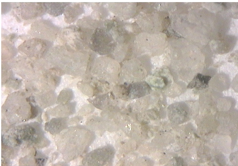
Figure 2. Sand grains from one of the Felix Jackson #62 samples (see text). The greenish grain near the center is ~300 microns long
