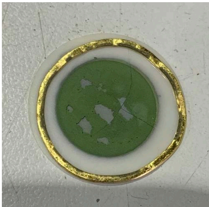
Figure 10.13 – Cell Removed from ProboStat with Gold Seal.
