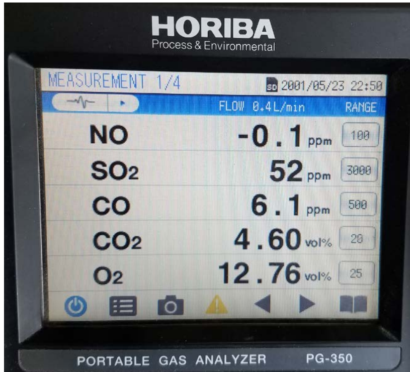
Figure 9.6 – PG 350 User Interface with MCFC Data.
