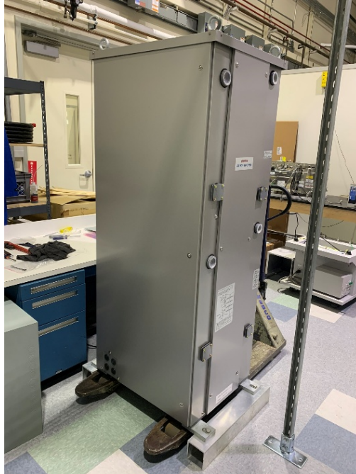
Figure 6.16 – Yazaki WFC-SC5 LiBr Absorption Chiller.
