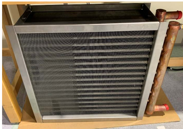
Figure 6.20 – Process Air Heat Exchanger.
