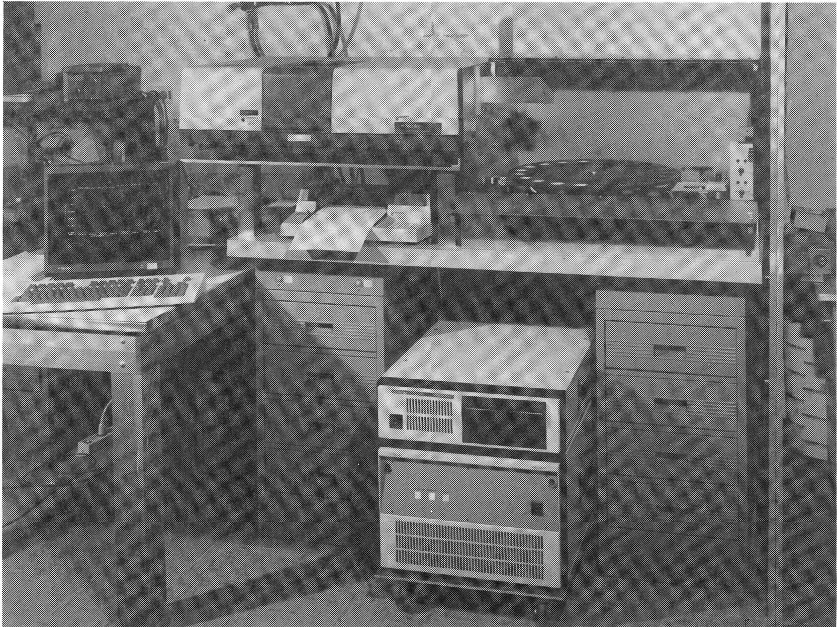
Fig. 4-1. Fourier transform infrared spectrometer and sample changer compartment.
