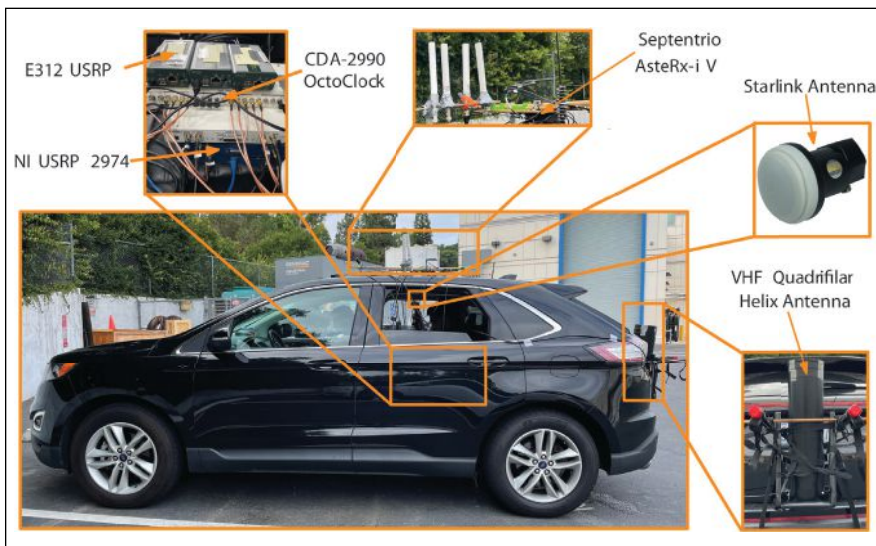
FIGURE 16 Hardware setup for the ground vehicle experiment.
