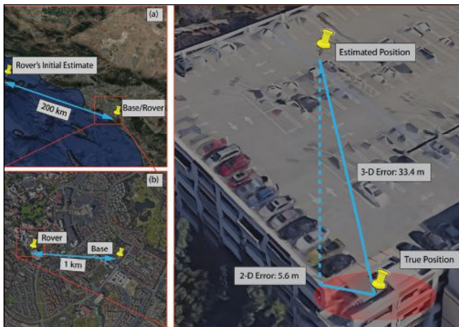
FIGURE 14 (a) Rover position initial estimate, (b) Base and rover true locations, and (c) True and estimated positions of the rover.
